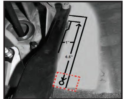
**Step 2.** Once the location of the hole has been marked, drill hole using an 11/16" drill bit or hole saw, drill the hole thru the fire wall. You will need to debur and paint the area around the hole to prevent rust.
