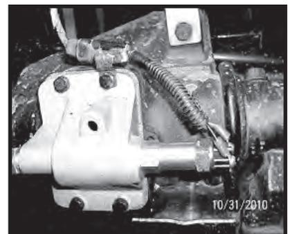
Step 9. You will need to trace the vacuum line back closest to the motor. Remove the vacuum line and cap off with the supplied rubber cap. Once the installation is complete, check for any oil or vacuum leaks. Test drive the vehicle and check for proper operation of the new cable lock kit.
