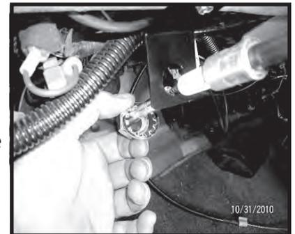
Step 4. Remove the factory actuator housing from the axle. Disconnect all vacuum lines and electrical connections. Remove the shift fork from the actuator housing. This can be done by removing the three E-clips that are attached to the mode shaft inside the actuator housing. When removing the shift fork it will be necessary to inspect for cracks or wear. If any damage is found on the shift fork it will need to be replaced for proper function and reliability. Item #450100 shift fork.
